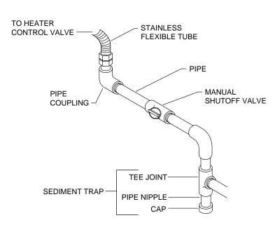
**IMPORTANT:** Loosen the pipe adapter on the flex tube before installing to the system piping.
